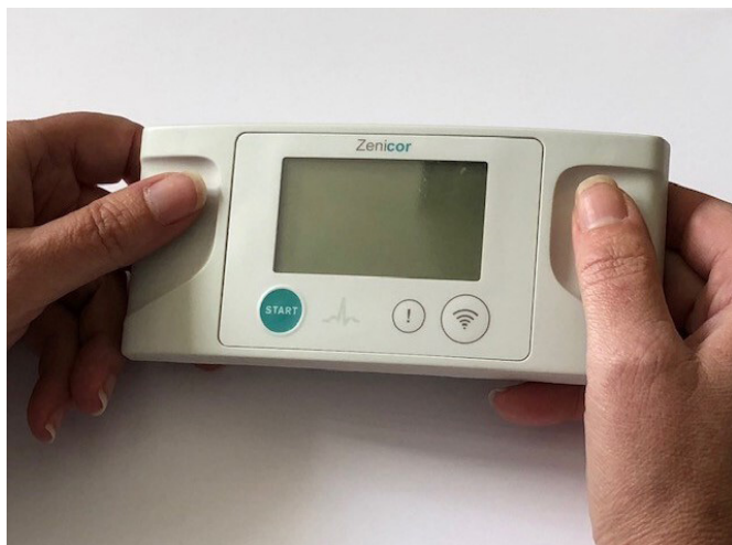
Figure 2 Zenicor hand-held ECG device used to screen for AF in the SAFER trial. AF, atrial fibrillation; SAFER, Screening for Atrial Fibrillation with ECG to Reduce stroke.
