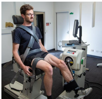
Figure SF3.3 Set up of knee muscle strength assessment using Biodex isokinetic dynamometer
